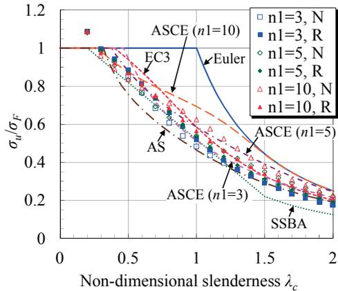
Fig. 3: Comparison of FE results with the EC3, ASCE, AS and SSBA design curves
