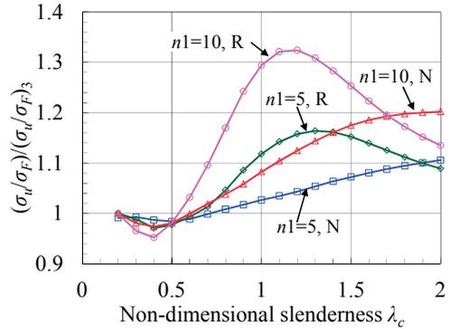
Fig. 2: Influence of strain hardening exponent  $n1$  on ultimate strength
