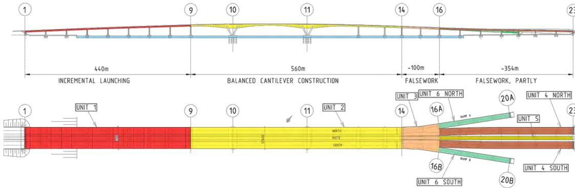
Fig. 2: Saadiyat Bridge – Elevation and Plan View
