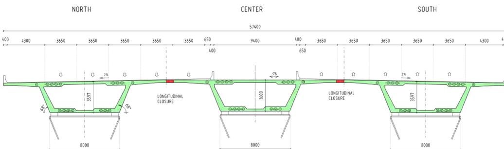
Fig. 3: Standard cross section Unit 1 – Incremental launching with transverse prestressing
