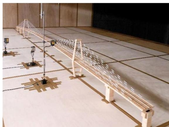
Fig. 3: Full aeroelastic model (S=1:150)
