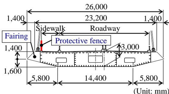
Fig. 2: Detail of stiffening girder (planned)
